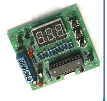
Ceramic Capacitors, Resistors, Push Buttons and Transistors should be easy to insert and solder into place! Make sure you follow the white outline or footprint of the PCB.
