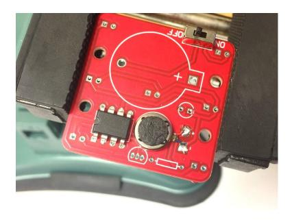
8) Place the resistor, transistor and the vibrator switch on the board and solder them. You can solder them one by one or all together.
