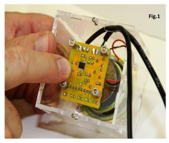
2. Refer to the enclosed PCB component layout diagram for the resistor value placement and the correct orientation for the electrolytic capacitors on the PCB and solder them in place.
