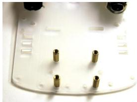
Step 10) Using the long screw and a Philips screwdriver, create a larger thread and fasten with a nut on the other side to the frame.
