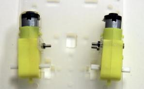
Step 5) (Optional) Slide in the encoders and glue the ends to prevent the encoder from falling out. This is entirely optional as most kits do not use the encoder function.
