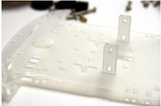
Step 4) This is what it would look like with both motors mounted into place. (Optional) If you want the motors to be positioned straight, align the motors as best as possible to be straight, flip the board and on the motor mounts insert inbetween the gaps some glue. Allow to set into place.
