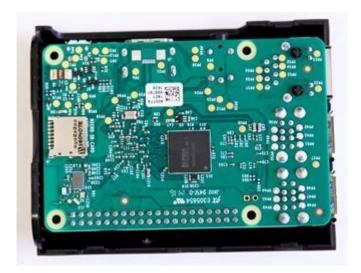
4) Place the top or bottom frame in and close the unit shut. Then on the bottom board insert four small screws to help secure the frame in place.
