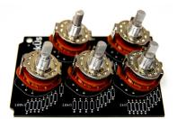
**9)** After placing all five of the POS into the board, flip the board and place the POS and board onto an even surface. This will allow you to solder the components in place easily.
