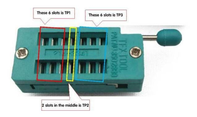
The test position of the patch element is on the right side of the test seat. There are above digital 1,2,3, each representative TP1, TP2, TP3. Test only 2 pin components, pin no test order, 2 pins arbitrarily selected 2 test points. 3 pin device pins are placed in the three test points, pin no test order. After testing, pin name of the element and the location of the test point be identified automatically and displayed on the screen.
