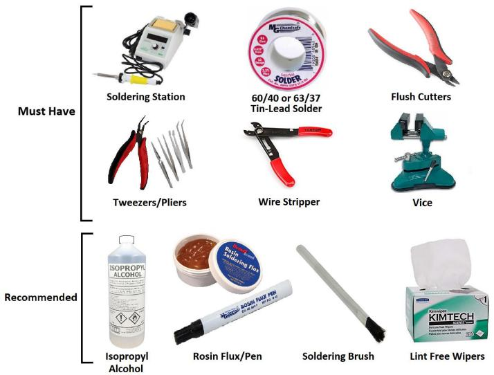
\*It is recommended to have some isopropyl alcohol and a fine soldering brush handy to clean off the excess flux on the circuit board when the soldering is done. \*ATTENTION\* DO NOT USE RUBBING ALCOHOL, IT WILL DAMAGE THE COMPONENTS.
