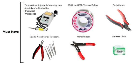
\*It is recommended to have some isopropyl alcohol and a fine soldering brush handy to clean off the excess flux on the circuit board when the soldering is done.
