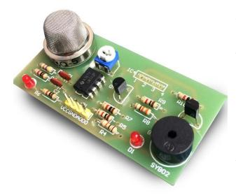
You may proceed to solder the blue potentiometer, then proceed to solder the black buzzer and the four-pin header.
