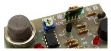
Option 2: As shown in the photo, solder the daughter board on the front side using the leads you placed aside from the LEDs. You will require a vice to help keep the components in place.
