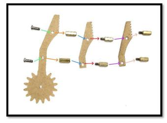
Now for the left gripper, proceed to mount as illustrated. The two small screw enter on the backside of the plate then the brass spacer fastens the standoffs. After fastening, you should repeat the process of layering the small claws with the spacers as shown in the image.
