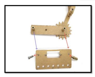
Before placing the servo bracket, observe two small screws located to the empty rectangular cut-out. You are recommended to place an MG-90 servo into that slot and fasten into place. Doing so at a later moment during the setup may be inconvenient for you. You may leave the white servo horn disconnect for now. Place the servo mount plate over the rectangular plate and fasten with the small brass M/F spacers and small screw. Place the final gear plate over the spacers
