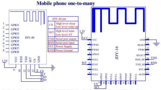
Mobile phone through JDY-16 serial port to JDY-40, and then through wireless transmission to over N JDY-40 modules
