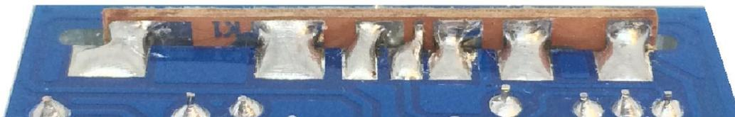
Use some thin wires or resistor leads to connect the two pads on the top side of the main PCB to the sound chip board.
