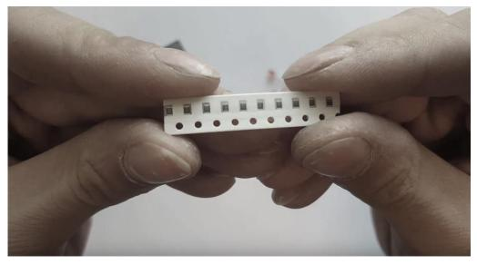
3) Take out the ICs, resistors and capacitors from their package by removing the clear tape and leave them on your workbench for the next step.
