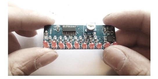
10) This kit provides a single row 2-pin header that can be used to power up the module. You can solder them if you have access to jumper wires or a pair of alligator clips. Otherwise, solder two pieces of wire to the positive (+) and the negative (-) leads on the board.
