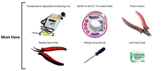
\*It is recommended to have some isopropyl alcohol and a fine soldering brush handy to clean off the excess flux on the circuit board when done soldering.
