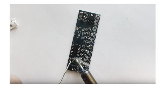
Once all the surface mount components are soldered on the board, proceed to the next step.
