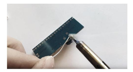
8) Insert the LEDs and solder the leads on the bottom side of the circuit board. You can secure the LEDs by taping them down on the top side of the board or by slightly bending their leads. You can solder them all at once or one by one.
