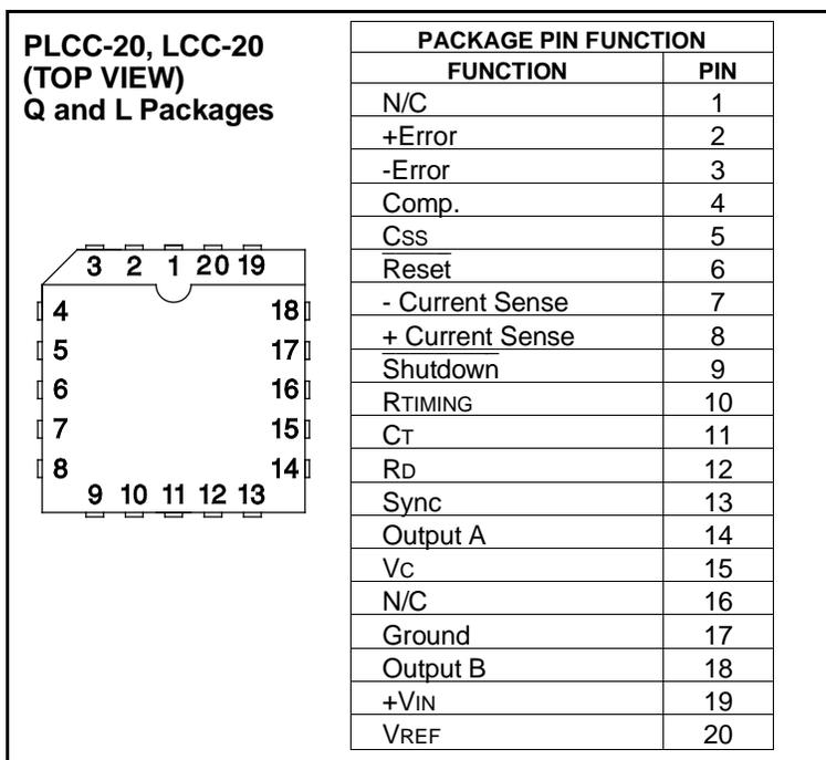
**ELECTRICAL CHARACTERISTICS:** +VIN = 15V, and over operating ambient temperature, unless otherwise specified, TA = Tj.
