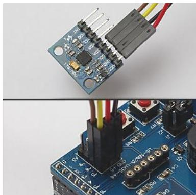
The multi-function shield does not expose the hardware I2C pins of some Arduino boards, such as the Leonardo. The following sketch uses the shield library to read raw values from the MPU6050 sensor, using either the Wire library or a software implementation of I2C. Download the full source code in order to upload the sketch to an Arduino, after which press button 1 on the shield to toggle reporting of sensor data, and press button 2 to cycle through acceleration, gyro and temperature values.
