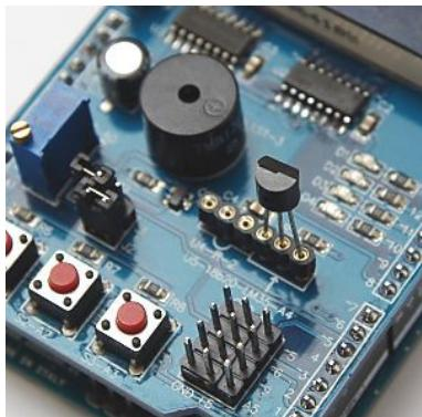
The multi-function shield has a socket for accepting an LM35 temperature sensor, which must be inserted correctly, otherwise you may irreparably damage your Arduino, or computer connected to it. You will know when the sensor is incorrectly connected, because it will become very hot. The multi-function shield library provides three levels of filtering for smoothing the readings from this sensor:
