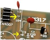
Solder the resistors in the correct order. 51k is identified as green, brown, black, brown, brown. Whereas 220 is identified as red, red, black, black brown. Solder the led with the flat side facing the opposite direction of the + symbol on the board. You can also identify it by looking through the led and locating the large plate as cathode (-). Solder the 10uF capacitor with the white band facing the white shaded region of the capacitor.
