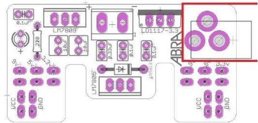
(Optional) Supply External Voltage from a wall power adapter that has a 2.1mm dc barrel jack connector with a maximum current rating of 1 amp and voltage rating of 35VDC.
