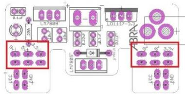
This region is where you required to insert a 2 pin shunt/jumper to supply the rail with your desired voltage.
