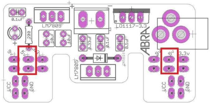
Placing jumper on 5v will allow the rail to be supplied with 5 volts to the entire rail, unless there is a break in the rail by default.
