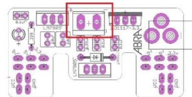
(Optional) Supply External Voltage from screw terminal block, pay attention to marking for polarity, with a maximum current rating for 1 amp and voltage rating of 35VDC from a bench power supply.
