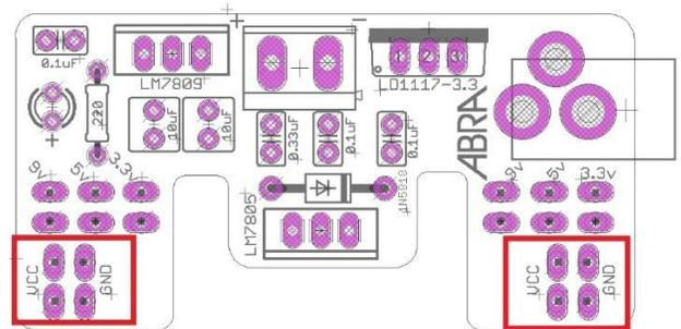
VCC voltage will be the output of what the jumpers for the rails are set as.
