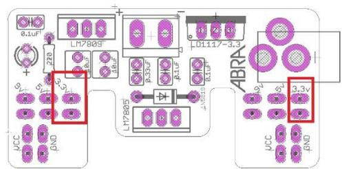
Placing jumper on 3.3v will allow the rail to be supplied with 3.3 volts to the entire rail, unless there is a break in the rail by default.
