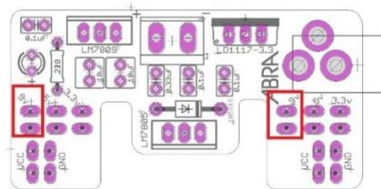
Placing jumper on 9v will allow the rail to be supplied with 8.2 volts to the entire rail, unless there is a break in the rail by default.
