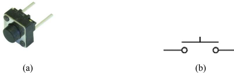
**Figure 0.7:** (a) Picture of a push button; (b) Circuit symbol for a push button.
