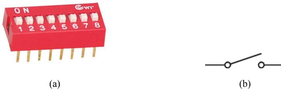
**Figure 0.5:** (a) Picture of an 8-input DIP switch; (b) Circuit symbol for a switch.
