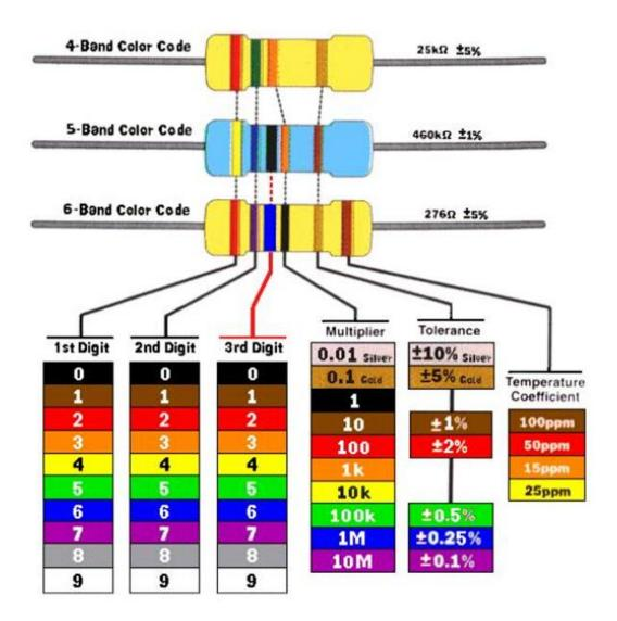
Resistors can have a different number of bands. Refer to the chart above to identify the value of your resistor. For example, [brown – black – black – red – brown] sequence of colors gives values [1 – 0 – 0 – 100 – 1%], which represents a  $10k\Omega$  resistor with 1% tolerance.
