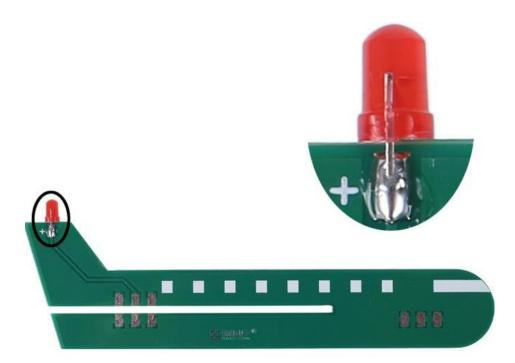
Step 17: Splice both PCBs and solder the connecting pads to secure the merge.
