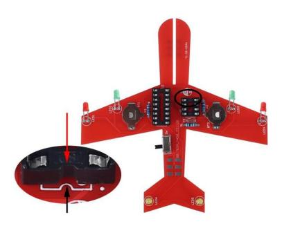
Step 13: 10uF Electrolytic capacitor at C1. Like the LED, the shorter pin is the negative. The side with the gray line also identifies the negative.
