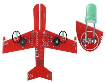
Step 8: Yellow LEDs at LED5 and LED6.
