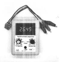
**8888 LED Digital Tube**: defined output voltage or electronics' reverse breakdown voltage
