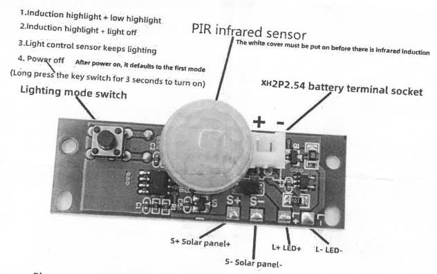
Please connect the battery first, then the LED, and finally the solar panel
