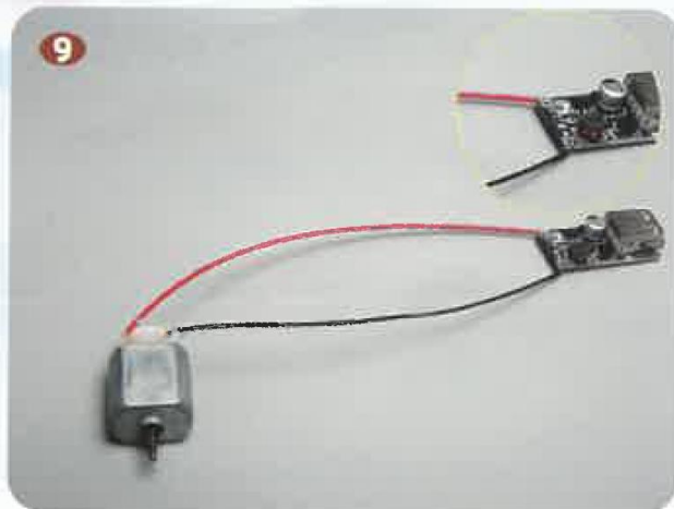
9 Connect the motor to the booster module using the wires as shown in the picture.
