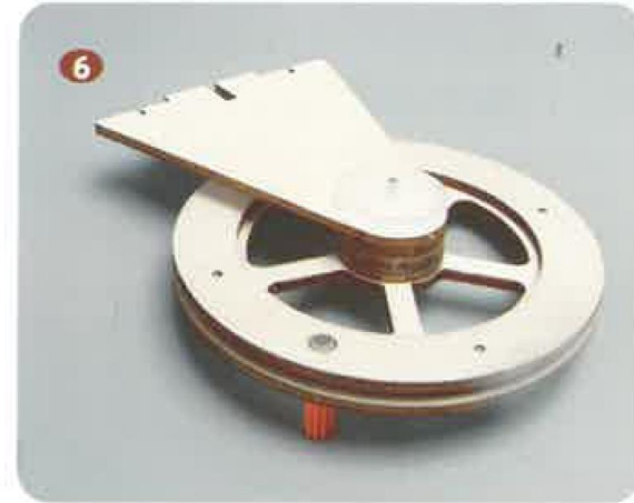
Install the large pulley as shown in the picture
