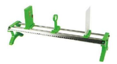
short focal length convex lens. The setup is as follows (using a dedicated F-shaped light source instead of candles):
