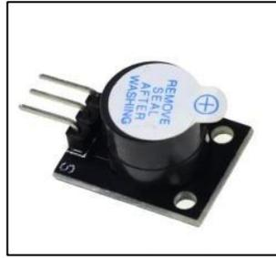
Buzzers are electronic devices supplied by power widely used in computers, alarms and printers that make sounds upon receiving current. This type of buzzer is active, meaning it contains an internal oscillating circuit that produces the sound, requires DC power supply (or a microcontroller pin that can carry that type of current), and its frequency and tone is fixed.
