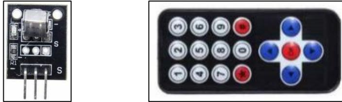
An IR receiver detects and decodes infrared signals sent by an IR emitter, which in this case is the remote control. They're widely used for wireless communication in television, audio equipment and electronics as such. Their common modulation frequencies are 36kHz, 38kHz and 40kHz.
