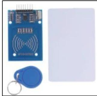
Radio Frequency Identification (RFID) encompasses technologies that use wireless communication between a tag and a reader to automatically identify and track objects. The transmission range of the tag is typically limited to a few centimeters from the reader. Most RFID tags have at least one integrated circuit (IC) and an antenna. The IC stores information and manages radio frequency (RF) communication with the reader.
