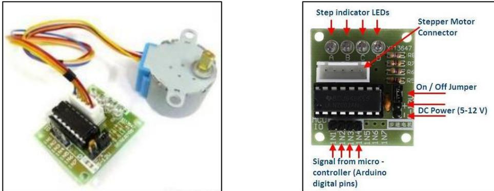
This four-phase (known for possessing four coils) unipolar stepper motor moves in half-step mode (8 steps per cycle) for precise motion. The four coils are labeled A, B, C and D. They are energized in the following order in their half-step mode:
