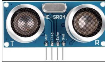
The ultrasonic sensor measures the distance between itself and the object using ultrasonic soundwaves through its two probes. One sends the ultrasonic waves and the other receives them and transforms the sending and receiving time into the distance. The sensor's detecting range is between 2 cm and 450 cm. The module uses ultrasonic transmitters, receiver and a control circuit. Its functionality is as follows:
