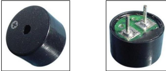
Unlike the active buzzer, the passive buzzer does not have an internal oscillating circuit and requires an AC signal to produce sound (a square wave). Its pitch is not fixed and can be controlled by frequency of input signal.
