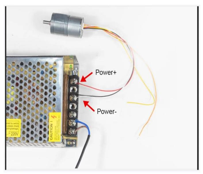
**Note:** it is not connected to the governor, but directly connected to the DC power supply. The red wire is connected to the positive electrode, and the black and white wires are connected to the negative electrode together.
