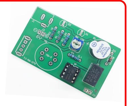
It is recommended to solder and cut of the excess lead with a flush cutter, one component at a time.
