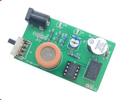
Insert the switch, DC connector and the MQ3 sensor as shown in the picture and solder them.
