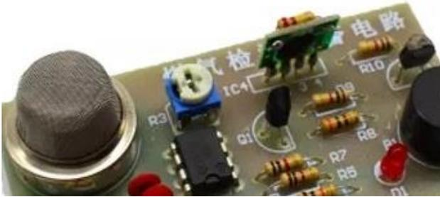
**Option 2:** As shown in the photo, solder the secondary board on the top side using the left over LED or resistor leads that you set aside from the previous steps. You will require a vice to help keep the components in place while soldering.
