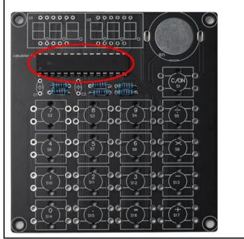
Step 4: Install the CR2032 battery holder at BT1, pay attention to the direction.
