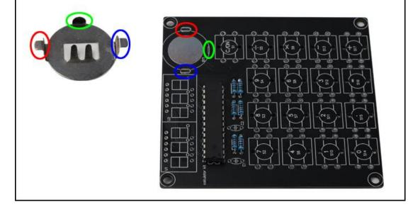
Step 5: After confirming the installation direction, straighten the pins of the CR2032 battery holder, insert them into the mounting holes, and solder one of the pins. After adjusting the position, solder the remaining pins, and the soldering is complete.
