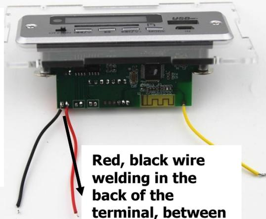
Red, black wire welding in the back of the terminal, between the solder joints must not be shorted
