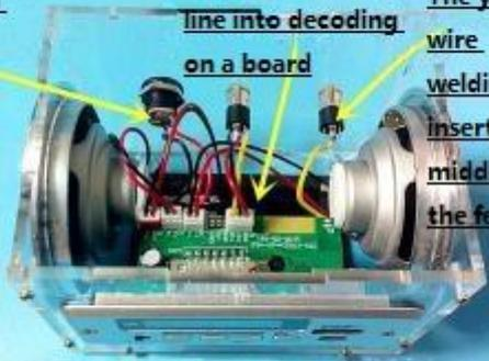
The third step: after the board with 2 \* 8 screws to the side panel and floor
