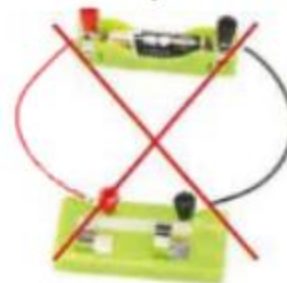
Figure 1-3: Wrong connection method. The switch is closed, causing a short circuit
