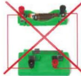
Figure 1-3: Wrong connection method, The switch is closed, causing a short circuit
