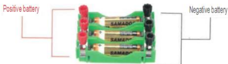
Figure 1-5: Battery series card connection
