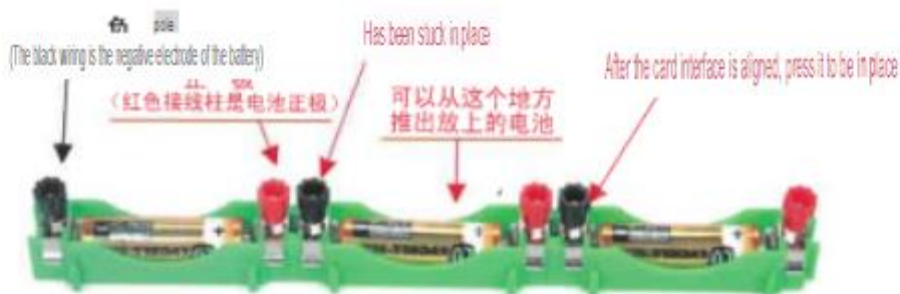
Figure 1-5: Battery series card connection
