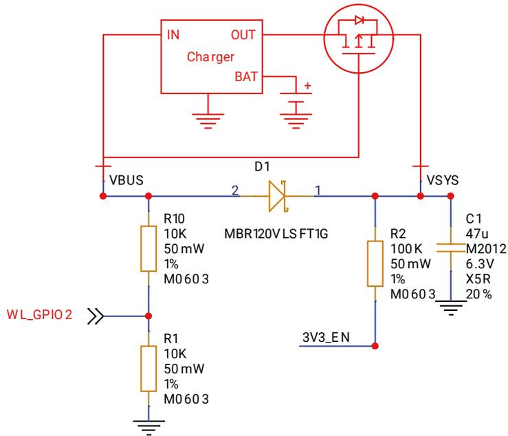
In the example we feed VBUS to the input of the charger, and we feed VSYS with the output via the previously mentioned P-FET arrangement. Depending on your use case you may also want to add a Schottky diode across the P-FET as described in the previous section.
