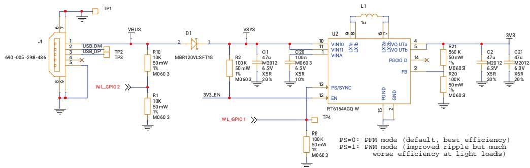
VBUS is the 5V input from the micro-USB port, which is fed through a Schottky diode to generate VSYS. The VBUS to VSYS diode (D1) adds flexibility by allowing power ORing of different supplies into VSYS.
