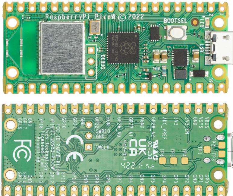
Raspberry Pi Pico W has been designed to be a low cost yet flexible development platform for RP2040, with a 2.4GHz wireless interface and the following key features:
