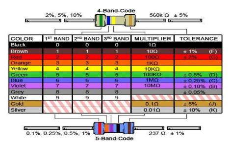
In resistors, there is always the first digit followed by the second digit followed by the third that is called a multiplier. For example, if we have Brown, Black and Red, the value of the resistor will be 10 multiplied by 100 which gives 1k, which is the resistor in our case.
