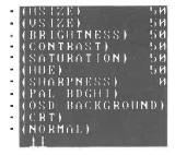
Horizontal size—Enter the menu after next by the up or down arrow key can be enlarged or reduced AV Horizontal size of the screen.
