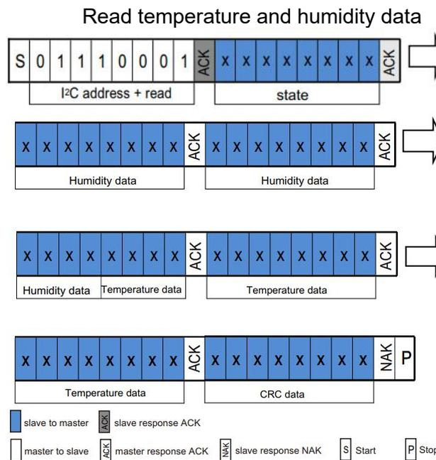
Note: The sensor needs time to collect. After the host sends a measurement command (0xAC), delay more than 80 milliseconds before reading the converted data and judging whether the returned status bit is normal. If the status bit [Bit7] is 0, it means that the data can be read normally. When it is 1, the sensor is busy, and the host needs to wait for the data processing to complete.
