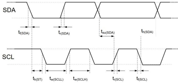
**Figure 9.** Timing diagram of digital input / output
