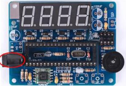
Step 15: Install 1pcs DC-005 Power Socket at 5V.
