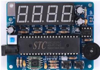
Step 20: Install 1pcs DIP-40 IC STC89C52. There is a mark on one end of the IC and there is a mark on PCB where the IC can place on. These two marks are corresponding to each other and are used to specify the installation direction of the IC.
