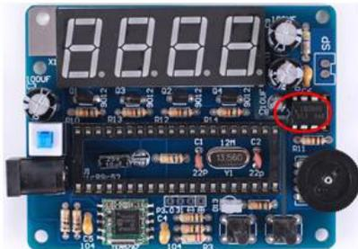
Step 19: Install 1pcs DIP-8 IC LM386. There is a mark on one end of the IC and there is a mark on PCB where the IC can place on. These two marks are corresponding to each other and are used to specify the installation direction of the IC.
