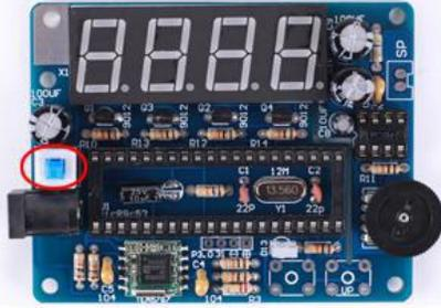
Step 17: Install 1pcs Self-locking Button at S4.
