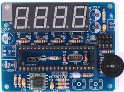
Step 14: Install 1pcs Red 0.56" 4Bit Common Anode Digital Screen at 056SMG\_4.
