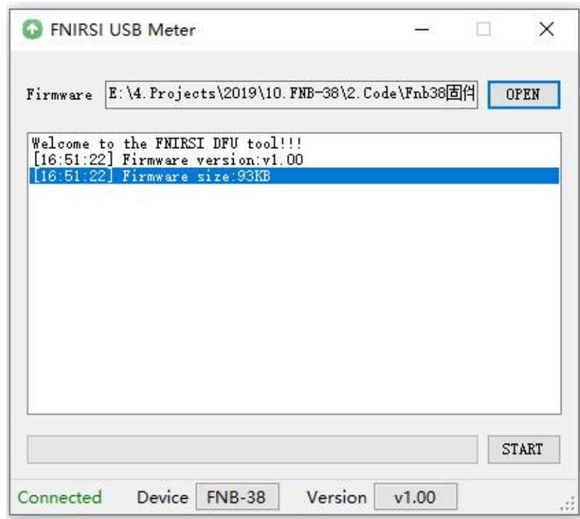
4. Click START to start upgrading the firmware. After the upgrade is completed, FNB38 will restart automatically.
