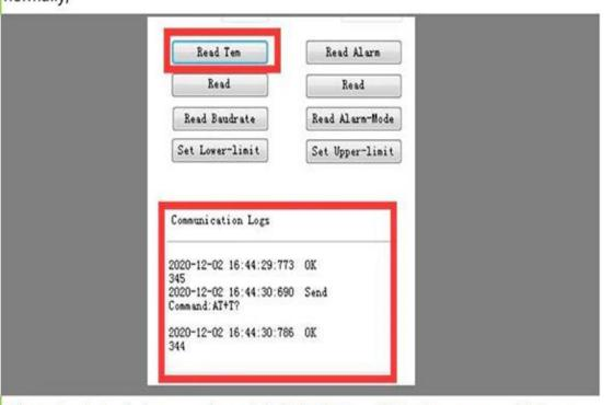
Select the desired alarm mode and click the button, fill in the upper and lower temperature limits (actual values), and click the set button to set the lower and upper temperature limits of the module.
