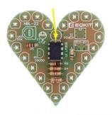
**Step4:** Solder S8050 at the labeled place on the board.
