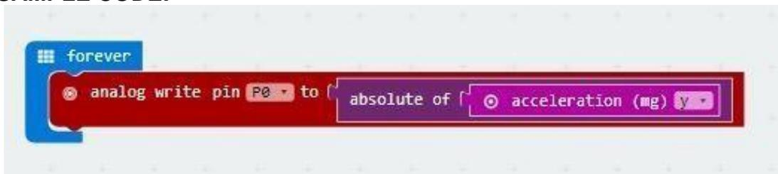
Figure 25 - Accelerometer Motor Control
