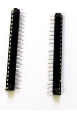
Take the 40 pin holder and break the middle bridge to create two strips of 20 pins. Solder the bottom socket in and flip the board.
