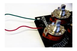
**14)** Repeat the same step from 12 for the secondary pad and use the black banana socket. Using a multi-meter test the decade resistance box, by turning clockwise you increase the value. By turning it counter clockwise you decrease the value (starting position). Place all switches back to starting position when you are done.
