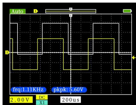
**11. Waveform screenshot:** Click in the button panel **SAVE** key, Capture the current screen and save. You can save up to 81 screenshots (9 pages in total, 9 per page), If there are more than 81 sheets, the oldest sheet will be replaced. You can delete unnecessary pictures.
