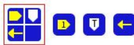
The first one is all, The following are vertical zero offset, trigger horizontal position, and trigger level. You can switch between these 4 options by moving the joystick up and down/left and right, press
