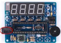
Step 15: Install 1pcs DC-005 Power Socket at 5V.
