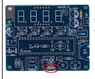
Step 2: Install 1pcs 220Kohm Metal Film Resistor at R3.
