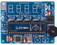
Step 10: Install 3pcs 0.1uF Monolithic Capacitor at C4,C5,C6.
