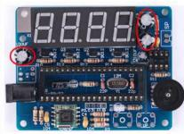
Step 16: Install 3pcs 100uF 50V Electrolytic Capacitor at C3,C9,C11. Pay attention to distinguish between positive and negative. The Longer pin is positive pole.
