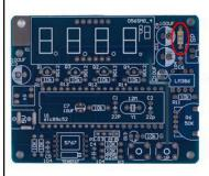
Step 1: Install 1pcs 4.7ohm Metal Film Resistor at R7.
