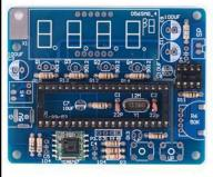
Step 8: Install 1pcs DIP-40 IC Socket at U1. There is a mark on one end of the IC Socket and there is a mark on PCB where the IC Socket can place on. These two marks are corresponding to each other and are used to specify the installation direction of the IC Socket.
