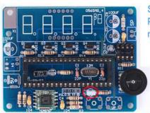
Step 13: Install 1pcs Blue 2\*5\*7 LED at D13. Pay attention to distinguish between positive and negative. The Longer pin is positive pole.
