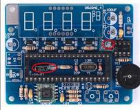
Step 12: Install 2pcs 10uF 25V Electrolytic Capacitor at C7,C8.Pay attention to distinguish between positive and negative.The Longer pin is positive pole.
