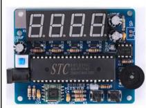
Step 20: Install 1pcs DIP-40 IC STC89C52. There is a mark on one end of the IC and there is a mark on PCB where the IC can place on. These two marks are corresponding to each other and are used to specify the installation direction of the IC.
