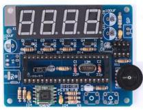
Step 14: Install 1pcs Red 0.56" 4Bit Common Anode Digital Screen at 056SMG\_4.
