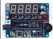
Step 19: Install 1pcs DIP-8 IC LM386. There is a mark on one end of the IC and there is a mark on PCB where the IC can place on. These two marks are corresponding to each other and are used to specify the installation direction of the IC.
