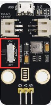
This is the switch. Slid to ON end, then the external lithium battery will be connected, supplying to the expansion board; on the contrary, slide to OFF, then the current of lithium battery will be disconnected.
