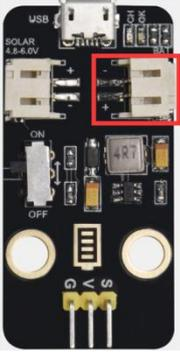
BAT, the output port of power, is interfaced with the lithium battery holder(rechargeable batteries) and saves the electric energy into batteries.
