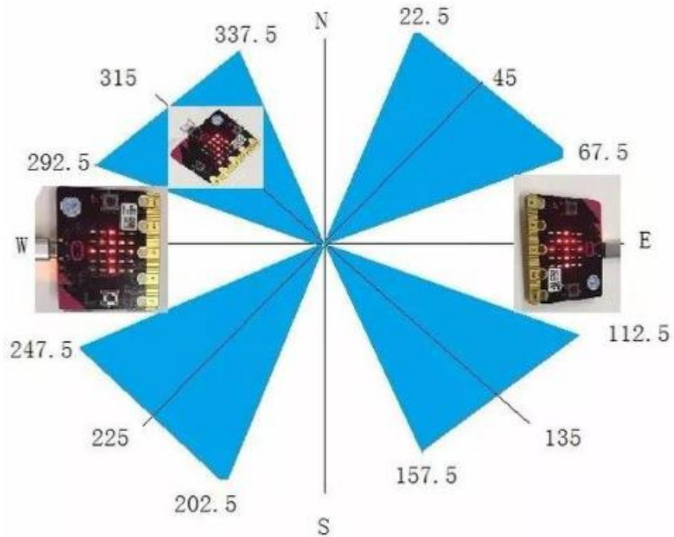
For the above picture, the arrow pointing to the upper right when the value ranges from 292.5 to 337.5. Because 0.5 can't be input in the code, the values we get are 293 and 338.
