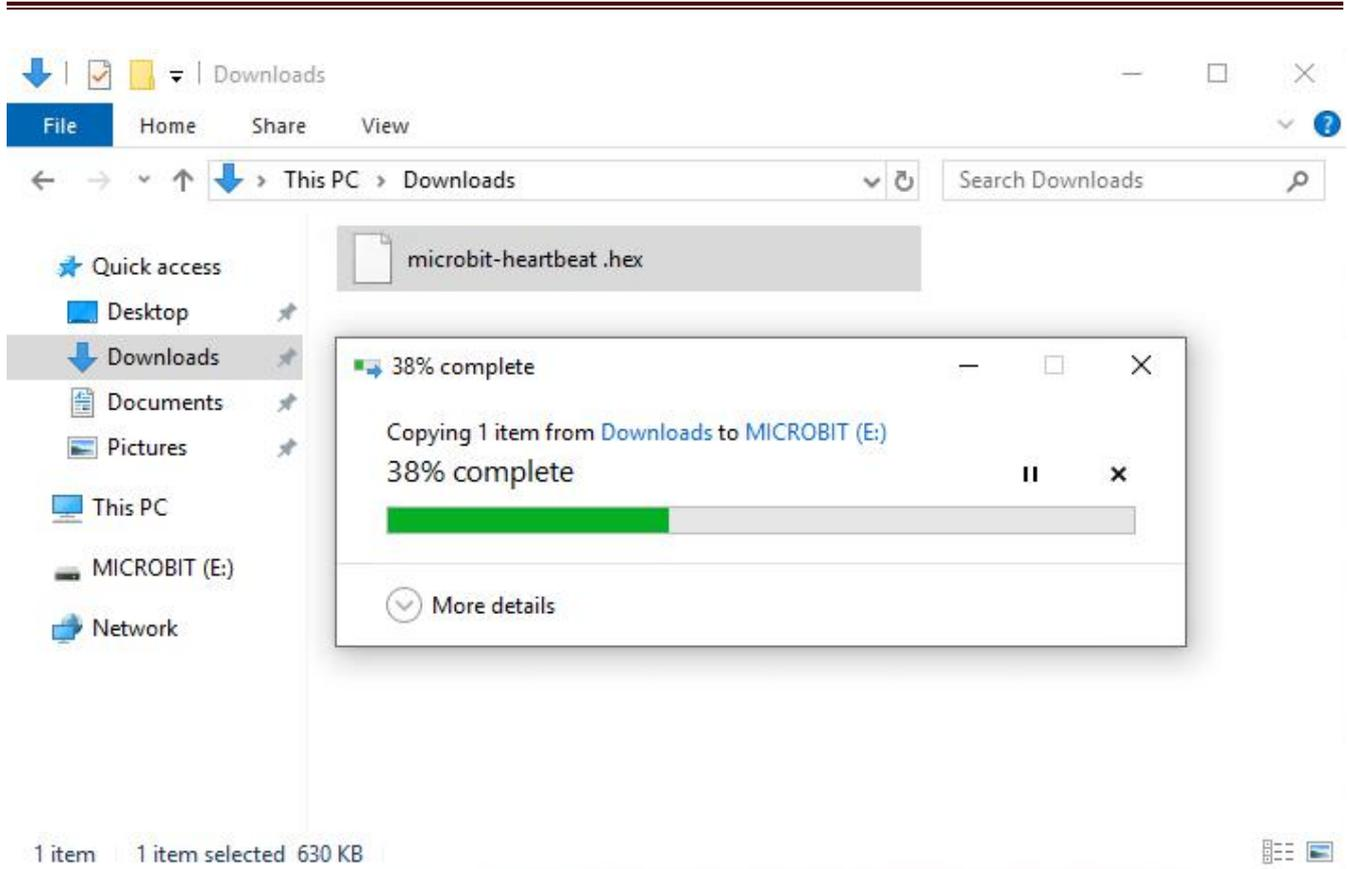
During the process of copying the downloaded hex file to the Micro: bit main board, the yellow signal light on the back side of the board flashes. When the copy is completed, the yellow signal light will stop flashing and remain on.
