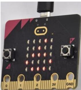
When the board is tilted to the right, the LED dot matrix displays the number 7 as shown below:
