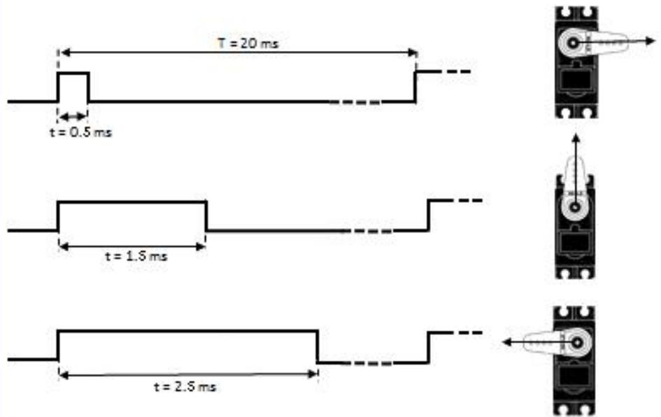
Through the experiment, the pulse range of the servo is 0.65ms~2.5ms.
