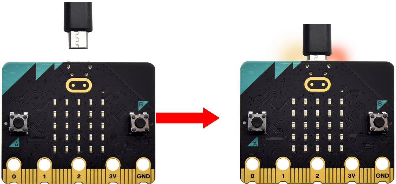
Secondly, if the red LED on the back of the board is on, that means the board is powered. When your computer communicates with the main board via the USB cable, the yellow LED on it will flash. For example, it will flicker when you burn a “hex” file.
