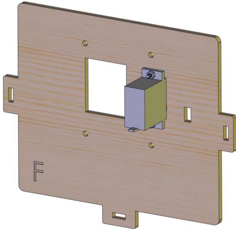
Adjust the angle of the servo controlling windows to 0°
