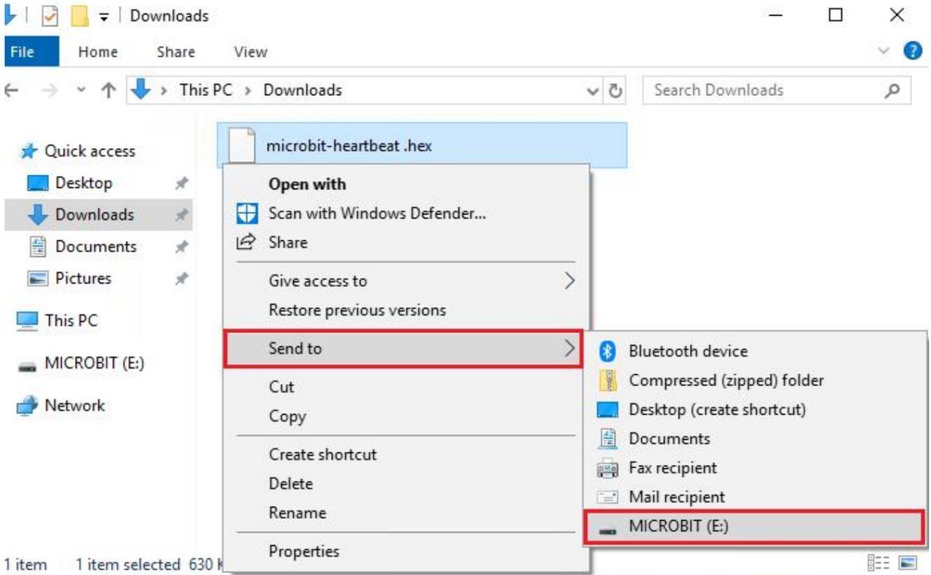
You can also directly drag the "hex" file onto the MICROBIT (E:) disk.
