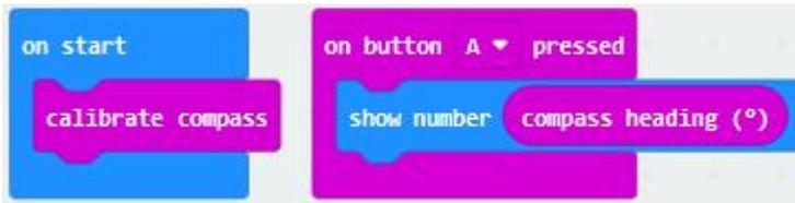
Note: it is imperative to calibrate the Micro:bit board for different geomagnetic fields existing in different places. And the system will make an automatic requirement if it is used for the first time.
