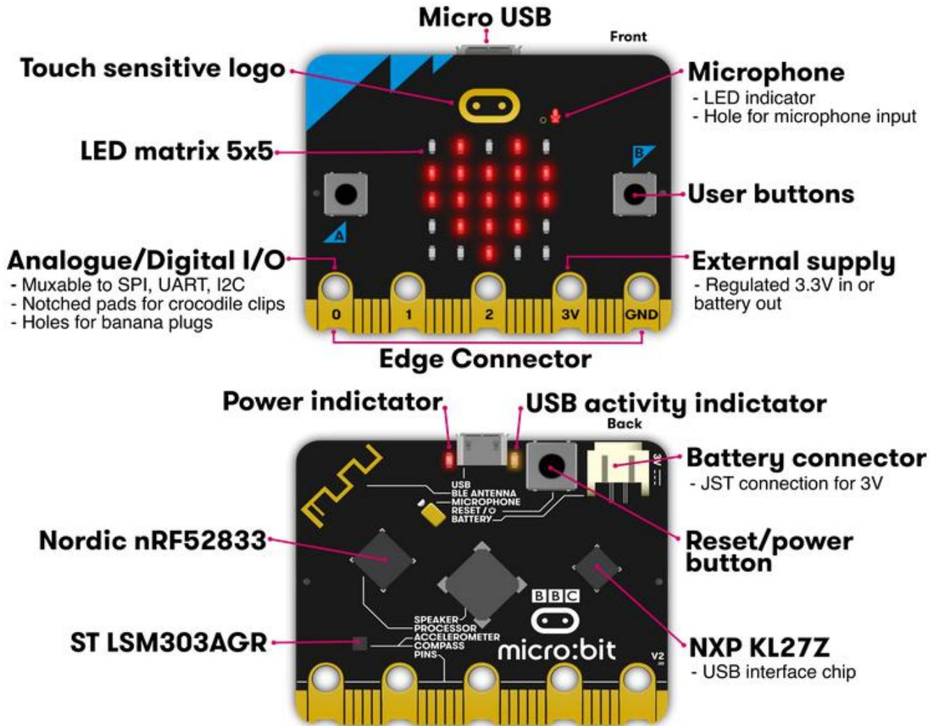
For the Micro: Bit main board, pressing the Reset & Power button, it will reset the board and rerun the program. If you hold it tight, the red LED will slowly get darker. When the power indicator flickers into darkness, releasing the button and your Micro: Bit board will enter sleep mode for power saving. This will make the battery more durable. And you could press this button again to 'wake up' your Micro:bit.
