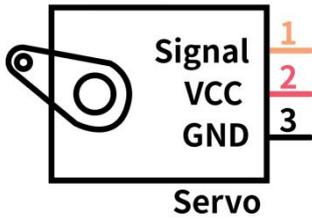
Servo motor is a position control rotary actuator. It mainly consists of a housing, a circuit board, a core-less motor, a gear and a position sensor. Its working principle is that the servo receives the signal sent by MCU or receiver and produces a reference signal with a period of 20ms and width of 1.5ms, then compares the acquired DC bias voltage to the voltage of the potentiometer and obtain the voltage difference output.
