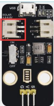
SOLAR4.8-6.0V, the input port of power, is connected to polar panels.
