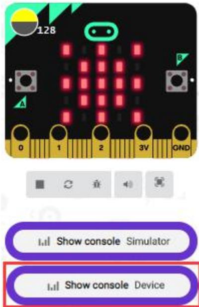
When the LED dot matrix is covered by hand, the light intensity showed is approximately 0; when the LED dot matrix is exposed to light, the light intensity displayed gets stronger with the light as shown below:
