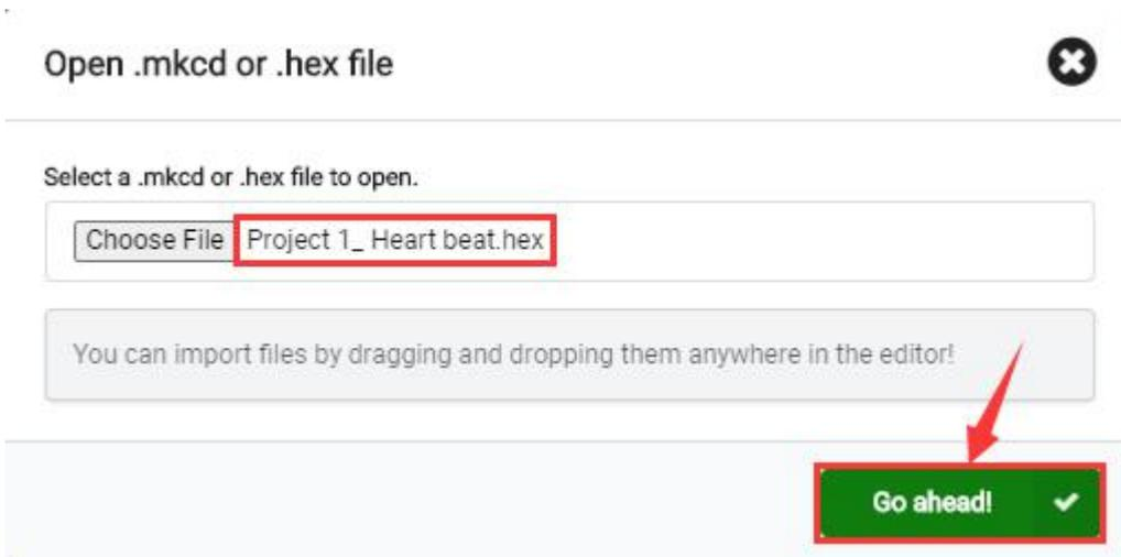
In addition to importing the test code file provided into the Makecode compiler above, you can also drag the the test code file provided into the code editing area of the Makecode compiler, as shown in the figure below:
