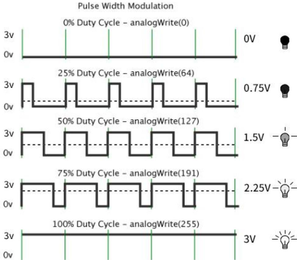
PWM is applied to light brightness adjustment, speed adjustment of motor and sound emitting.
