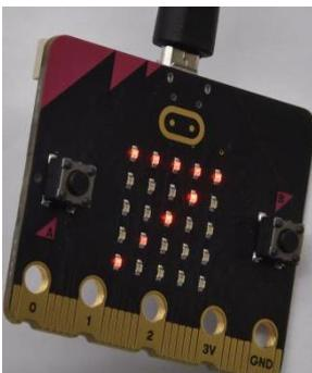
When the board is knocked to the floor, this process can be considered as a free fall and the LED dot matrix shows the number 8. (Please note that
